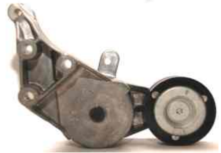
V03, Tensor correa Poli v VW Golf IV 1.9 SDi motor AGP, AMT
